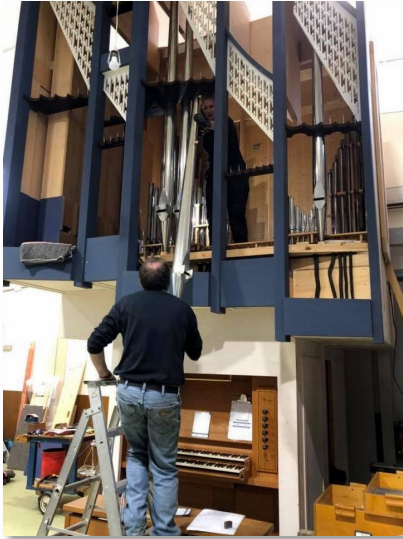
Mike and Lisa installing the Pedal Gemshorn 8' pipe.
